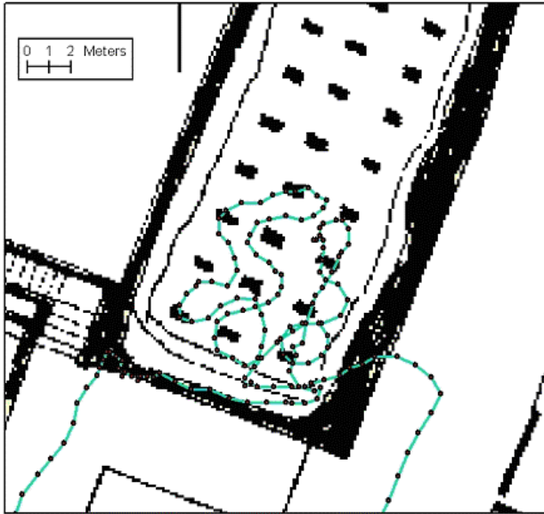
Fig. 8 – A complex path surveyed by BT-GPS EMTAC
